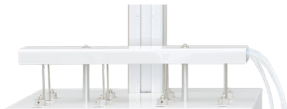
Automated sampling station ASS-9 on top of a DT from the DT 950 series
